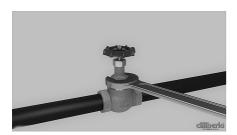
To assemble the bonnet on the valve body it is advisable to tighten it gradually to prevent the seal between the two parts from being subjected to excessive stress.
