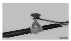
After installation, it is good practice to record the tightening of the bonnet and gland nut. In case of leakage from the stem, simply tighten the gland nut with a spanner.
