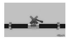
Never use ball valves to regulate flow, but only to intercept fluids to intercept fuids, so to avoid damages to gaskets.
