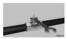
When leaking from the stem, remove the handle by unscrewing the nut and fasten the gland screw. If leaking continues, take off the gland screw and check the PTFE stem gaskets.
